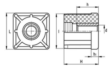
d = M12 h = 10 H = 38 h1 = 8 Internal tube size = 31.0 I = 31.0 L = 35 Outer tube size = 35
